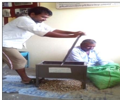
Inclined concave opening (Refined Groundnut decorticator)
