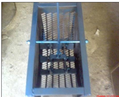
Inclined concave opening (Refined Groundnut decorticator)
